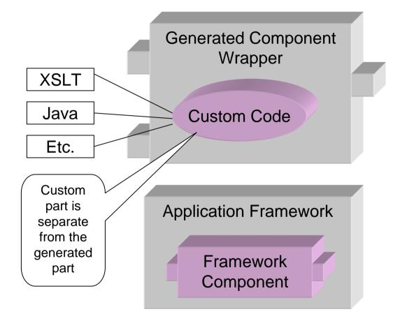
Application components provide service implementations with user supplied logic. These "plug into" the users architecture as composite application components
